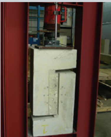
Longitudinal shear test arrangement with Eazistrip cast into one side of the joint. The load was applied by jack through the test frame.
